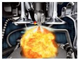
Second to oil pressure, exhaust gas temperature (EGT) may be the most critical operating parameter on your diesel engine, because excessive EGT can bring a host of problems that fall under the meltdown category, both figuratively and literally. Every material has a melting point, some lower than others, and when things get too hot, expensive parts within or attached to your engine start welding themselves together or disintegrating into the exhaust pipe.
