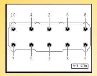
IMPORTANT: ALL BOLT THREADS, BOLTHEADS AND WASHERS MUST BE LIGHTLY OILED.
