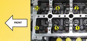
IMPORTANT: ALL BOLT THREADS, BOLT HEADS AND WASHERS MUST BE LIGHTLY OILED.
